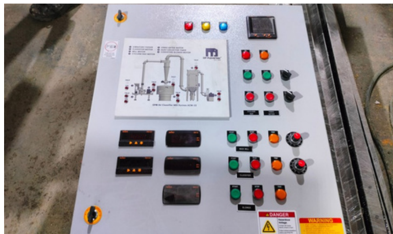
▶ Typical control panel with process flow diagram
