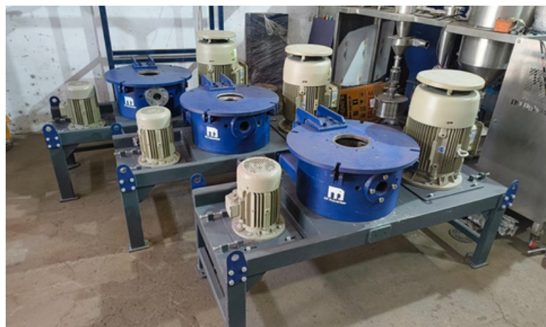
► Production of 3 nos. DP® ACM-15 for grinding of organic yellow pigment
