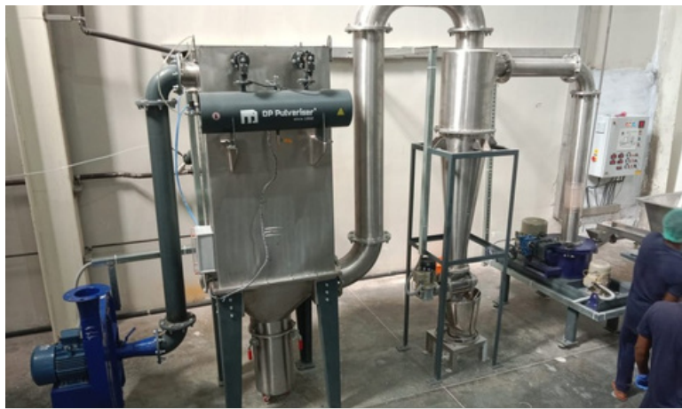
► Installation of DP® ACM-10 in South India for grinding of coconut flakes
