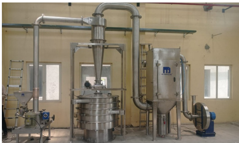
► Installation of DP® ACM-10 in North India for grinding of biomass
