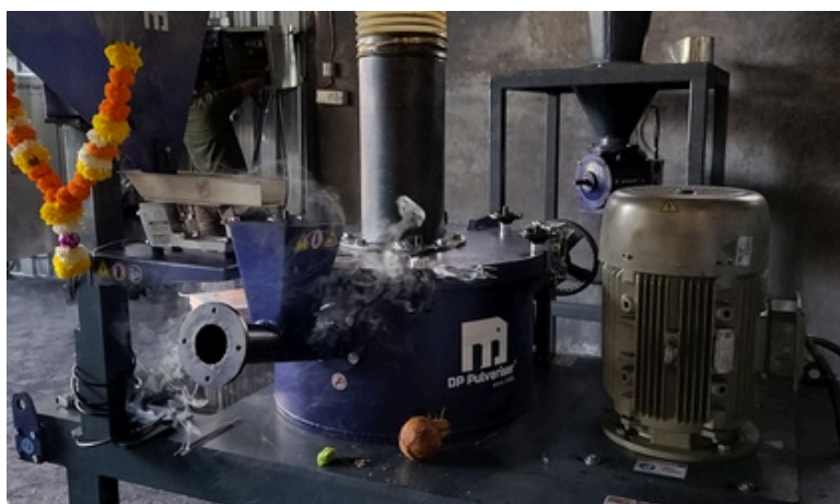
► Installation of DP® ACM-30 in West India for grinding of synthetic graphite
