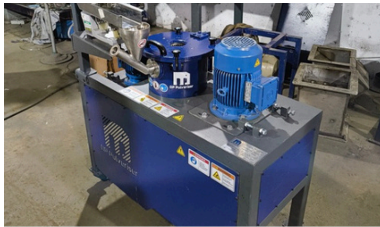
► DP® ACM-2 Air Classifier Mill Lab-Pilot Size
