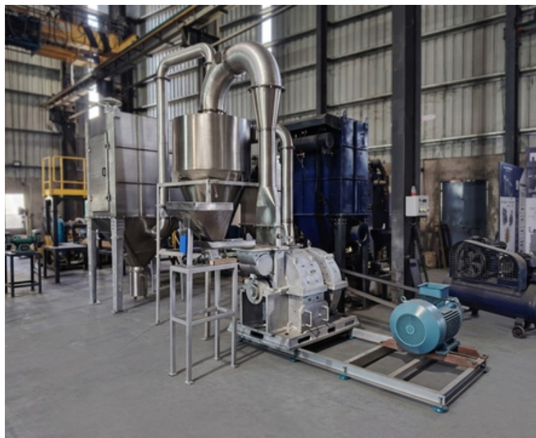
▶ DP® IP32 Broad Chamber Impact Pulveriser for Grinding of Dehydrated Onion at Customer in Mahua, Gujarat
