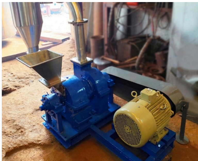
▶ DP 8 Mini Impact Pulveriser for Crushing of Manganese Ore in Zambia, Africa
