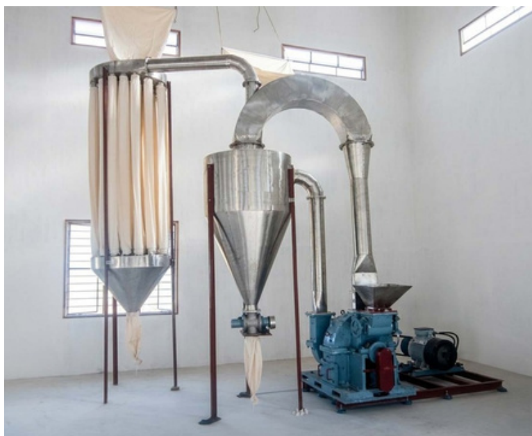
▶ DP® IP32 Impact Pulveriser with SS304 Contact Parts
