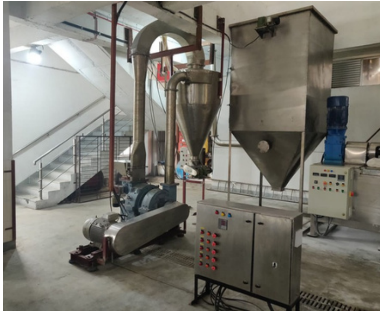
▶ DP® IP25 Impact Pulveriser with SS304 Contact Parts
