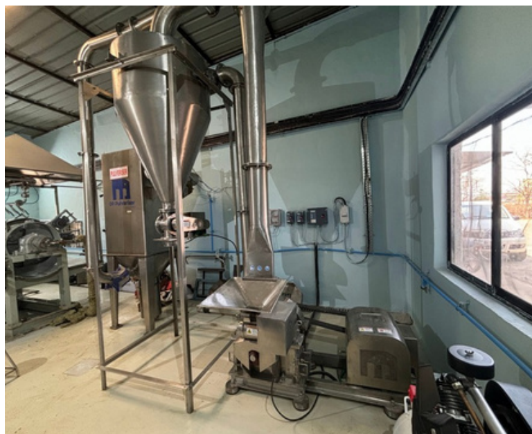
▶ DP® IP20 Impact Pulveriser SS316-SS304 MOC at leading food ingredient manufacturer in Mumbai
