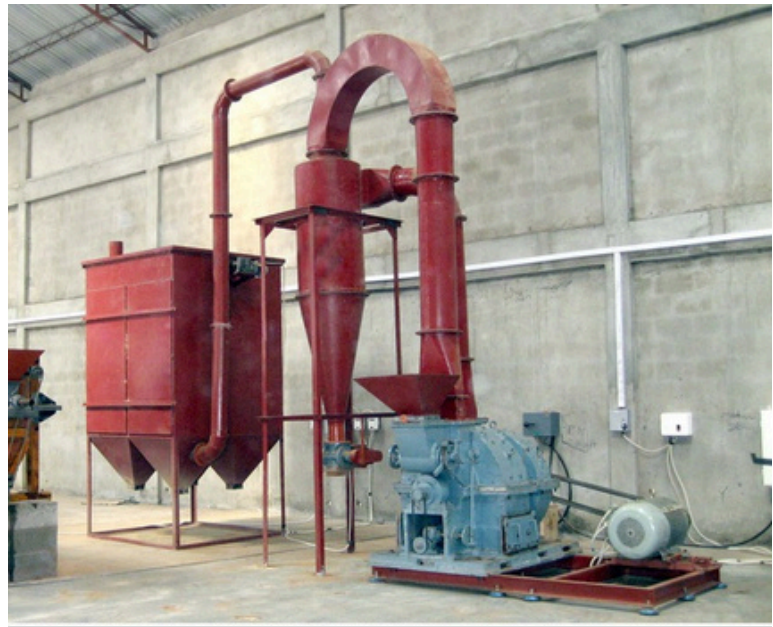
▶ DP® IP42 with Close Dust Collector and RAV in Ghana, Africa
