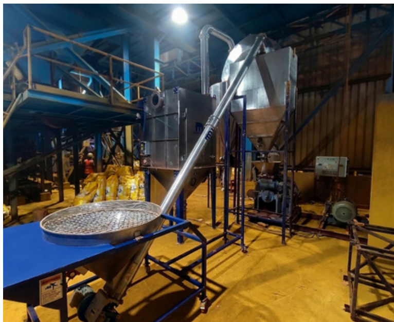
▶ DP® IP32 Impact Pulveriser for grinding of Pigment at large Indian MNC at Jamshedpur, Ranchi
