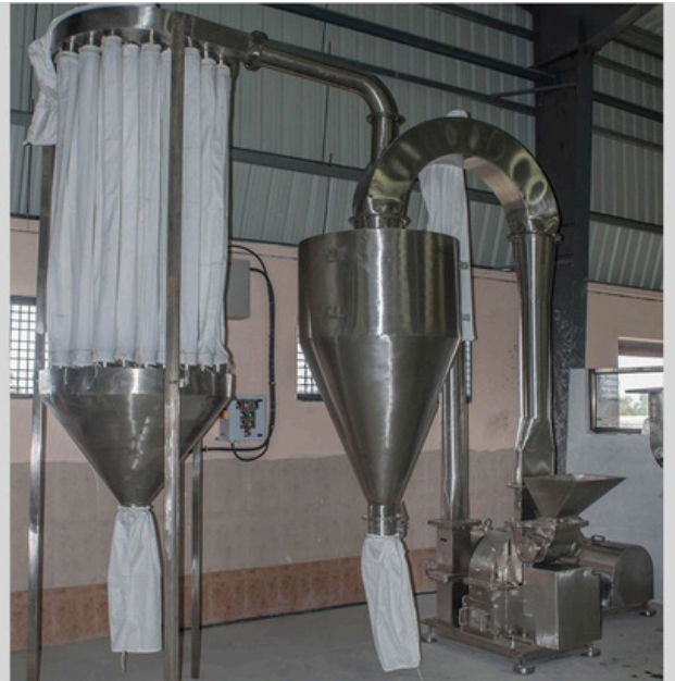
▶ DP® IP25 Impact Pulveriser in SS304
