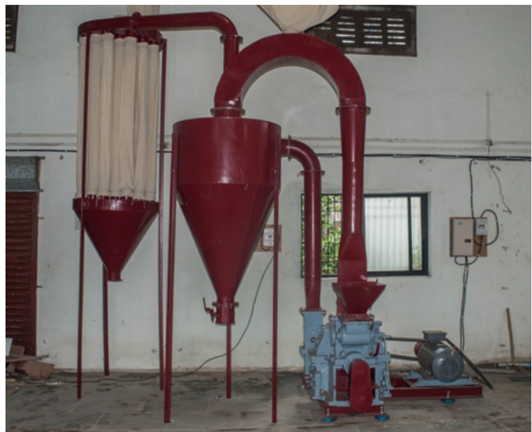
▶ DP® IP20 Impact Pulveriser at Nickel-Al Manufacturer in Vapi, Gujarat
